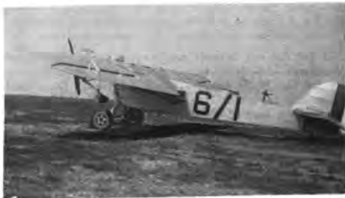
First monoplane in the U.S. Navy [ Martin VO-5 ] Hampton Roads 1925. Note generator on top fuselage. (Koterba Photo)
